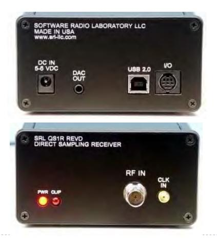
much promise. It covers DC-62 MHz (or up to ~500 MHz when oversampled) with up to 2 MHz bandwidth. The QSIR interfaces to its PC by USB. The entire design and all its support software is "open" licensed.
